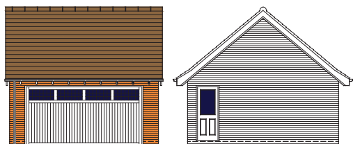
Detached Double Garage - Front and Side Elevation
